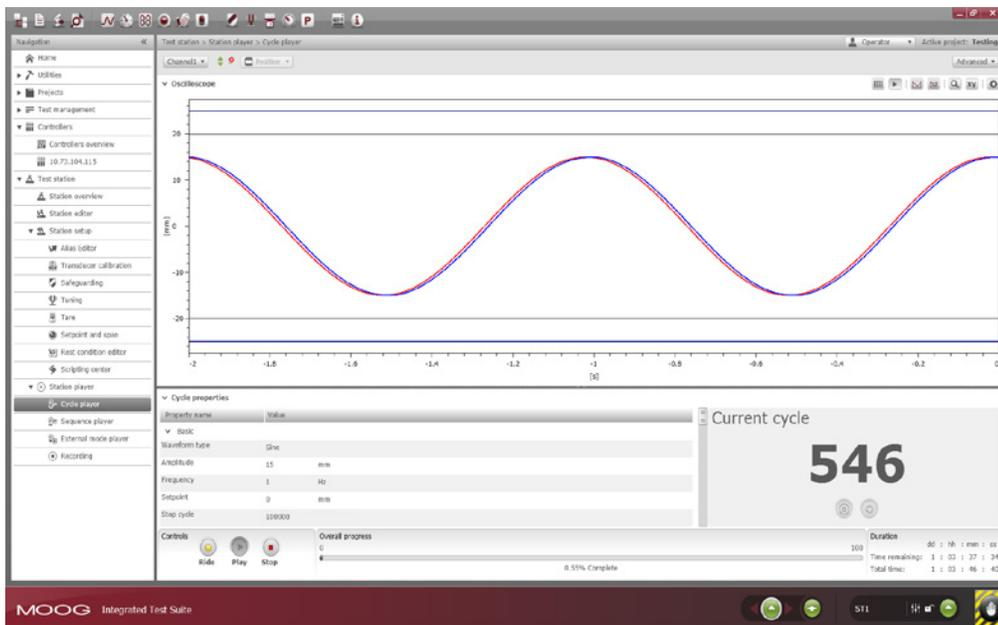
The Cycle Player puts all necessary information on one screen to command and monitor a cyclic test. Amplitude and phase matching controls automatically adjust the command signal to achieve targeted waveforms.
