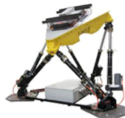
The Hydraulic Simulation Table provides acceleration or displacement inputs to reproduce time history data collected on proving grounds. Test samples generally include body mounted components or systems like EV batteries, engine mounting systems, cooling modules or cockpits.
