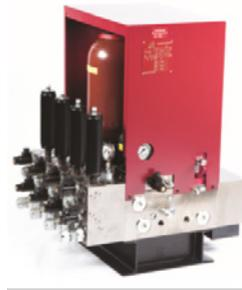
The Moog Hydraulic Service Manifold (HSM) provides on/off hydraulic pressure with an adjustable transition from off to high pressure. Filters protect sensitive servo valves and accumulators provide instantaneous flow or pressure damping when needed. Several flow-rating sizes with 1 to 4 station options are available.
