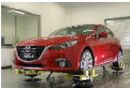
Our Four Poster Test Systems include hydrostatic bearing test actuators for low friction, high velocity and high side load carrying capacity. Our systems are found in research labs where they are used for ride quality assessment and Noise, Vibration and Harshness (NVH) testing. They're used in durability test labs to validate selected body, chassis, and suspension designs. They are also used in production facilities to assess squeak and rattle concerns.
