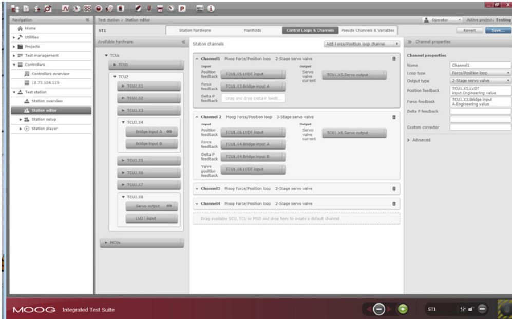
This is the central place to configure the station hardware and software. The user adds specific hardware I/O, creates logical channels and desired control loops, and can add pseudo channels for calculations.
