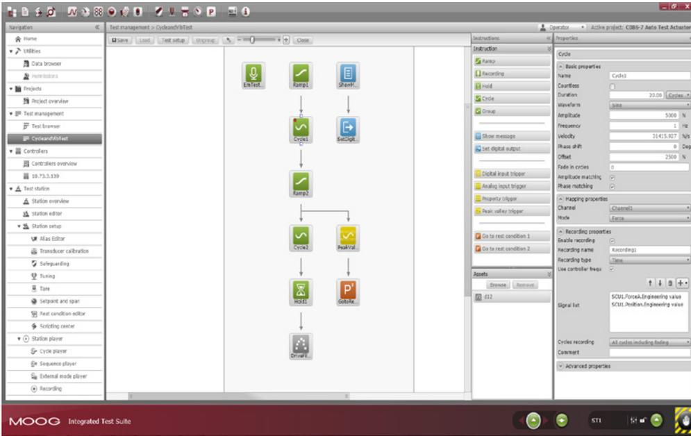
The Test Builder allows the user to quickly create and/or edit test definitions. Tests consist of instructions, actions, triggers, or assets like drive files. These instructions include items like ramp, recording, cycle, or grouping for nesting instructions.
