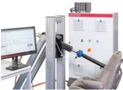
For design and production verification, Moog Electric Multi-Axis Test Systems are designed for efficient operation in a range of static or load/deflection tests to cyclic loading with test specimens like seat systems or door closures. These quiet systems are plug-in ready and have a lower total operating costs than equivalent hydraulic systems.
