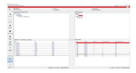
The final stage in the test setup is to define the test spectrum. This is accomplished by pressing the -Define Spectrum- button. Here the user can customize the test profile in detail.
