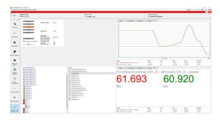
The test creation is now complete and the test is ready to run, this is accomplished by pressing the -Operate Test - button. The operator screen in the top left window can be used to go online and initialise and run the test. The graphs on the right hand side can be configured to display commands and feedbacks so that the operator can monitor the test.
