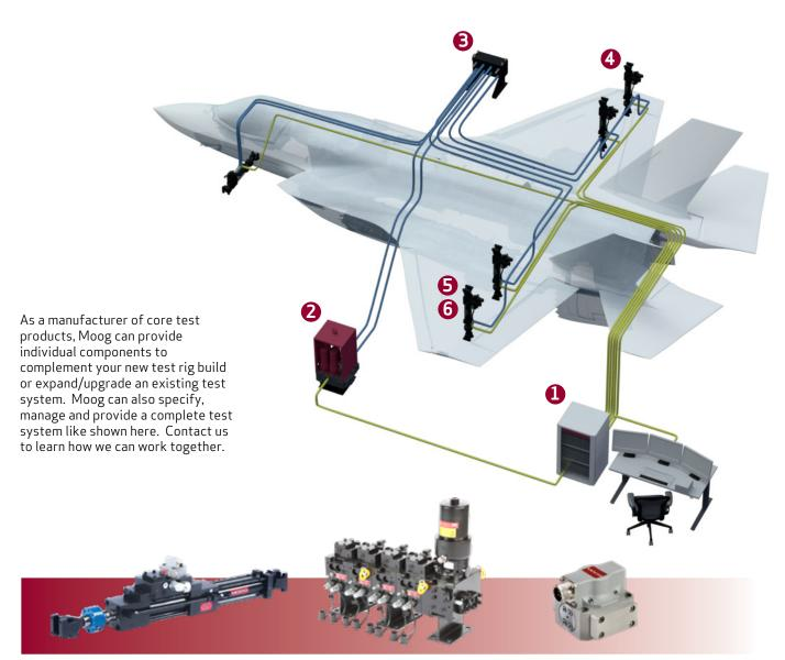
4 HYDRAULIC TEST ACTUATORS Choose from a family of fatigue-
