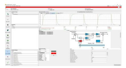
The operator can now tune each channel in the test by pressing the –Tune Controllers - button. The channel can be selected from the left hand window. Select each channel in turn and the relevant tuning parameters, function generator and feedback parameters are displayed in the window, along with a graphical representation of the control loop to give the user an understanding of the control loop configuration.
